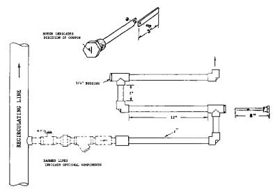
The Corrosion Rack illustrated here is a piping installation for water flow that is designed to be used for corrosion measurement. The right angle turns of this rack are designed to insert corrosion coupon holders. These holders ordinarily consist of steel or other threaded plugs with a Teflon® holder. To the end of this holder, a Corrosion Coupon is attached using a Teflon® screw and nut combination. A flow restricting orifice or flow rate indicator is used to simulate a critical flow rate.
